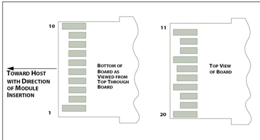
Figure 2 SFP28(56) Module Contact Assignment
