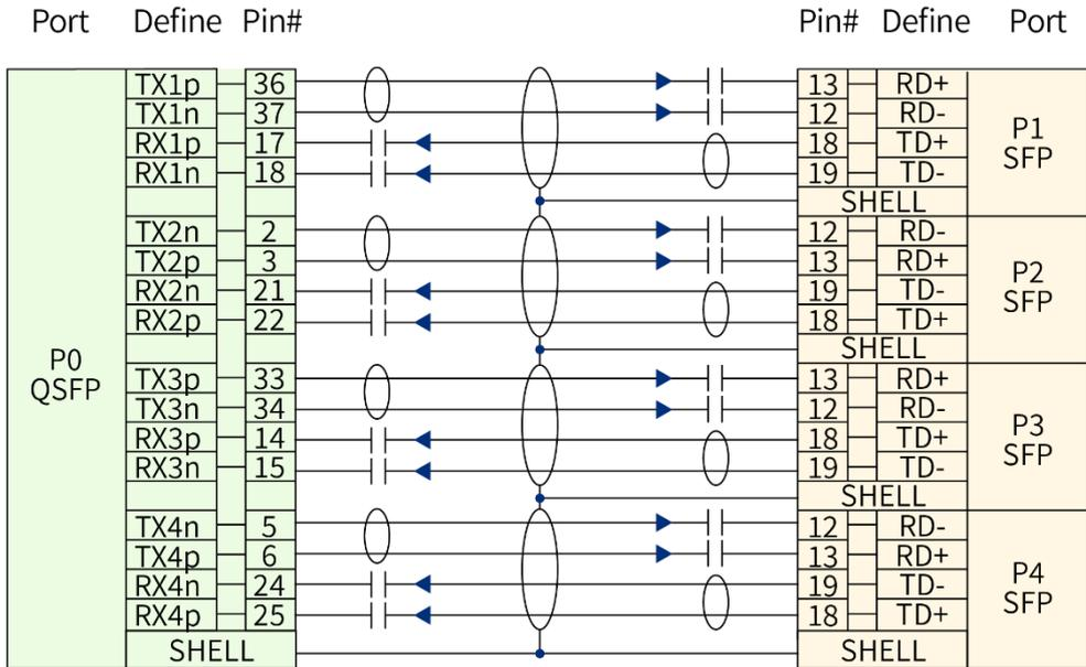
Figure 3 QSFP28(56) to 4\*SFP28(56) Direct Attached Cable Assembly Wiring
