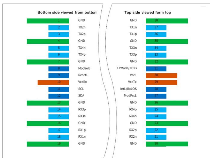
Figure 1 QSFP112 Module Contact Assignment
