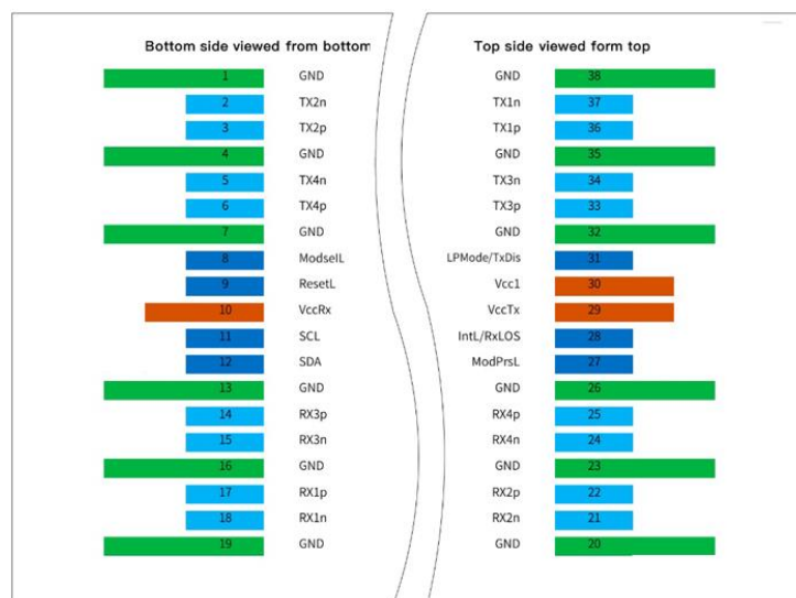
Figure 2 QSFP112 Module Contact Assignment
